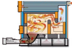
RRF – Solid retort burner with underfeed stoker auger
